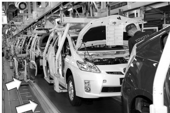
indexed final assembly line at Toyota
